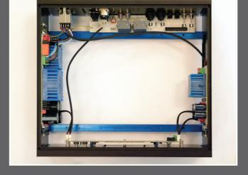
We have no output buffer or filter at the DAC output providing the cleanest possible output signal, just a transformer matching the impedance of the converter resistors to the outside world and isolating them from external infruence.
