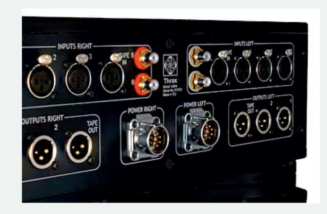
DHT tubes require a lot of auxiliary electronics for optimal operation, so in this case we have split the unit in two parts. A power supply and the active unit. This keeps all mains AC and rectifier noise in a separate box while final regulation and filtering is still done next to each element in the amplification circuit. Everything is microprocessor controlled and the unit's status is displayed on a large color LCD visible from your seat.
