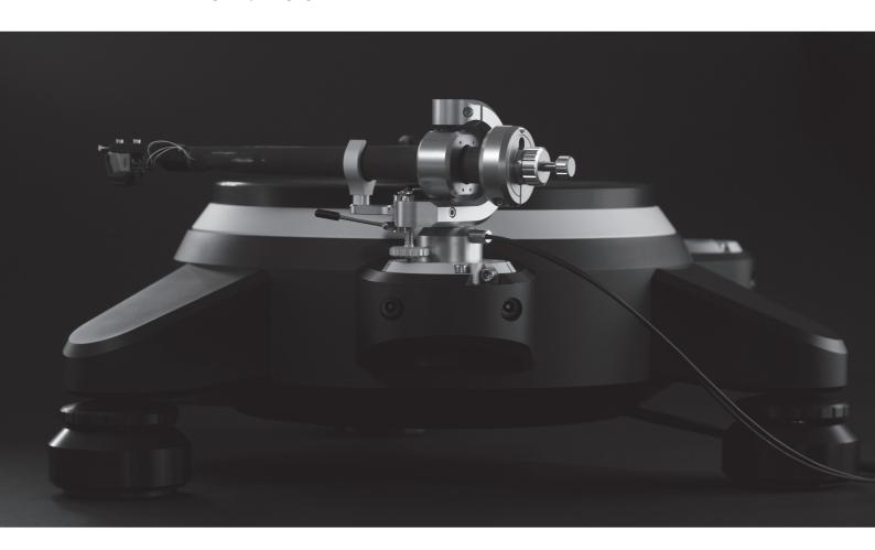
The XD1 Record Player System is delivered with a unique and exclusive arm - the CF1-Ti series. Available in 9 and 12 inch versions. This new arm is a special edition of the CF1 series that incorporates an internal titanium tube under the carbon fibre laminate for an even higher stiffness. The headhsell frame is also machined from titanium instead of stainless steel as on the standard CF1 series.
