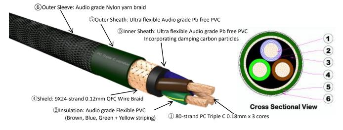
All metallic parts are treated with the \*FURUTECH lpha (Alpha) Process (Super Cryogenic & Demagnetizing Treatment.)
