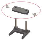
2. Loosen support fixed screws and then remove support unit.
