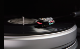
Boron Cantilever with Micro-ridge stylus
